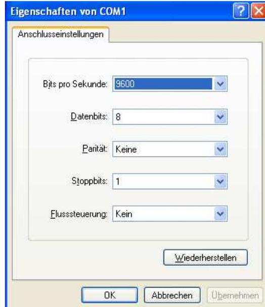
Sensor can be used with commercially available terminal-software (e.g. Hyper-Terminal)
